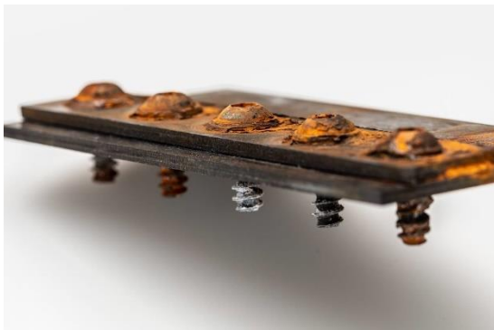
Figure 3a: Exemplary CFRP components with conventional steel screw for direct screw connection after a 720-hour salt spray test
