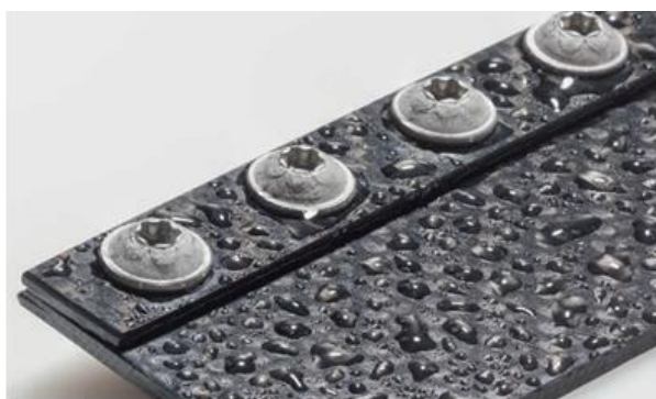
Image 3b: Exemplary CFRP components with b&m CARBONPLAST® screw for direct screw connection after a 720-hour salt spray test
